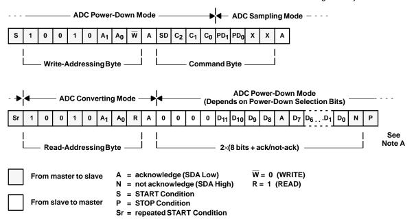
NOTE: (A) Use repeated START to secure bus operation and loop back to the stage of write-addressing for next conversion.
