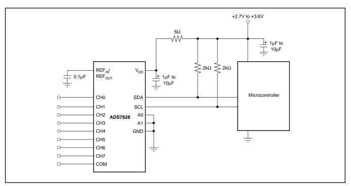
FIGURE 1. Basic Operation of the ADS7828.
